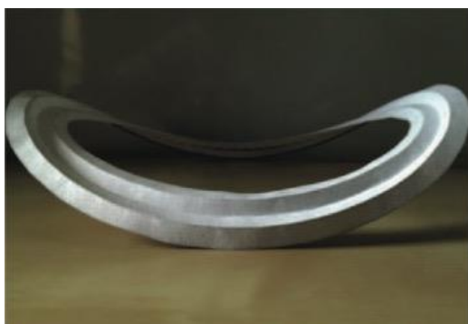
Fig. 6. Curved fold origami structure with three prescribed curves, in [5]
