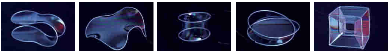
Fig. 14.23 Minimal surfaces in form of soap films (images courtesy of K. Rittenschober). Minimal surfaces are characterized by vanishing mean curvature.
